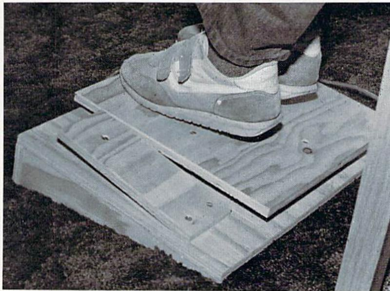
Figure 5 Foot joystick in action
